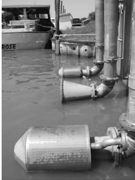
Figure 4-3 Two test screens (near and far), with control intake (mid) used in EPRI wedgewire screen testing.
