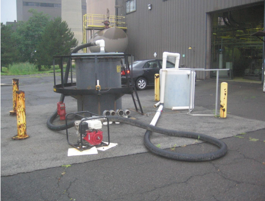
Figure 4-1 Net-in-barrel collection system (white polyethylene barrel) in use at discharge seal well of generating facility.
