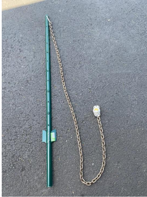
Figure 13 Stake & chain deployment apparatus for KLO stations.
