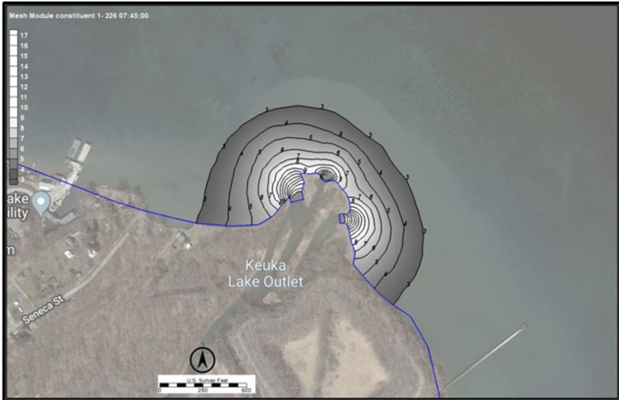
Figure 4-25 \Delta T Contours for Scenario Simulation 2 at 8/14/21 07:45. The enclosed area where \Delta T is \geq 3^\circ\text{F} is 16.4 Acres
