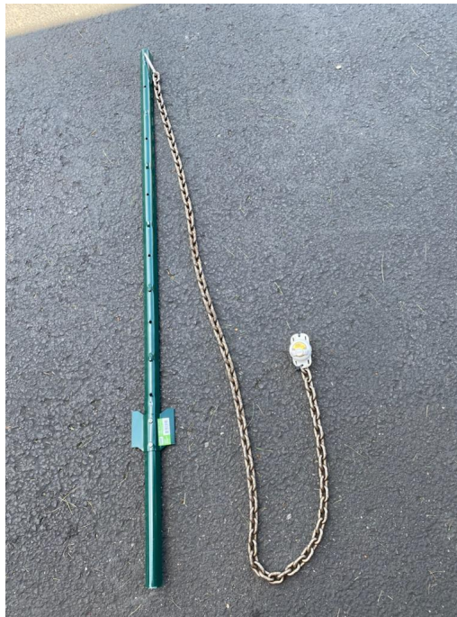
Figure 3-1 Attachment of HOBO sensor to chain and metal fence post.
