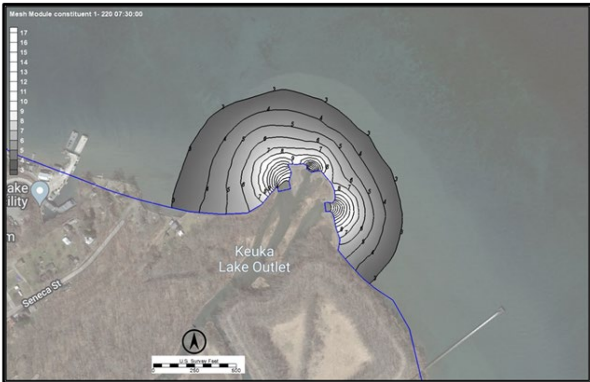
Figure 4-26 \Delta T Contours for Scenario Simulation 3 at 8/14/21 07:45. The enclosed area where \Delta T is \geq 3^\circ\text{F} is 18.7 Acres
