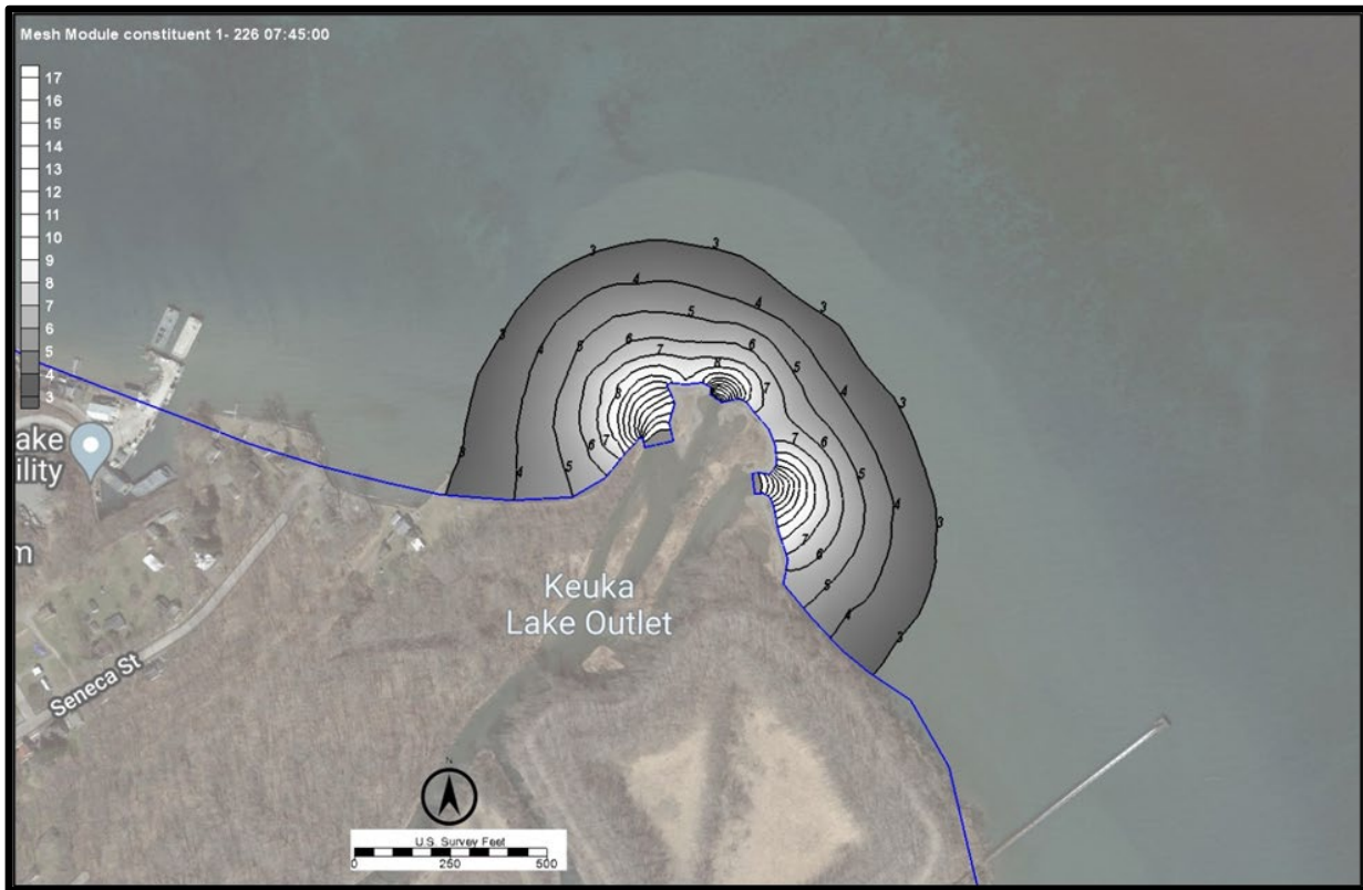
Figure 6.10: \Delta T Contours for Scenario Simulation 8 at 8/14/21 07:45. (Background Air Temp also increase by 6 Degrees F). The enclosed area where \Delta T is \geq 3^\circ\text{F} is 15.5 Acres
