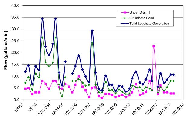
FIGURE 3-1: MEASURED LEACHATE FLOW RATES
