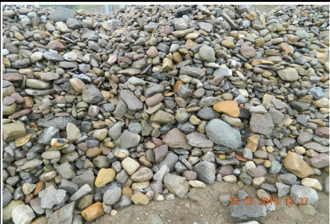
Photo 27: Light Stone Fill stockpile (10/3/16)
