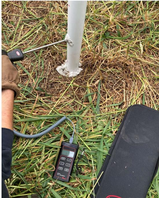
Photo #4 - Sample Point LW2 Gas Flow Sampling
