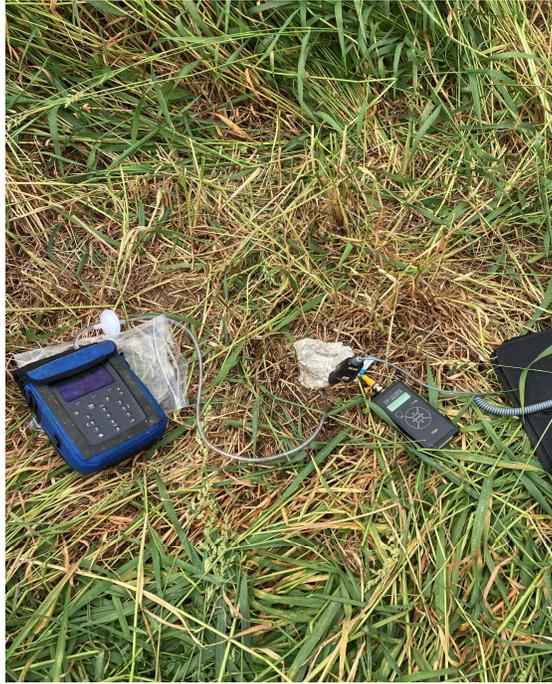
Photo #3 - Sample Point LW2 Gas Composition Sampling
