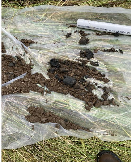
Photo #2 - Sample Point LW4 Soil/Waste Characterization During Augering
